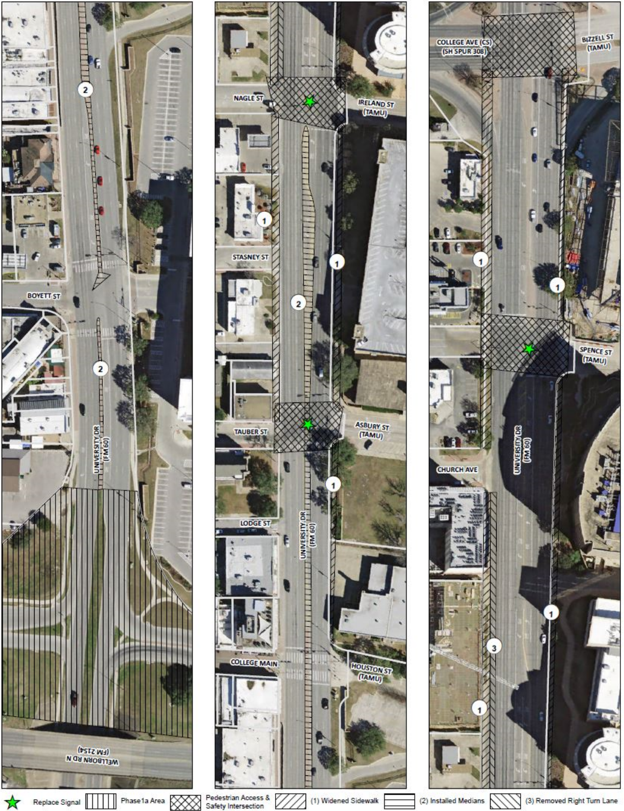
Figure 3 – Phase 1A and 1B Improvements of University Drive (FM 60) from Wellborn Road (FM2154) to College Ave (SH SPUR 308).
